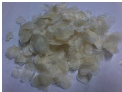
Figure 1: Optical image of as-received fish scales (FS) of Rohu fish before pyrolysis
