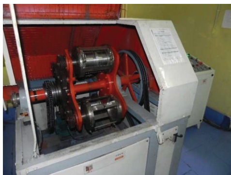
Figure 1: Dual-drive ball milling
