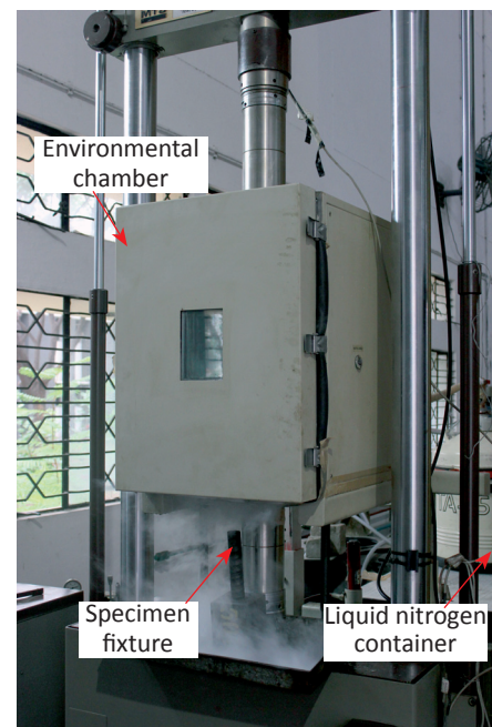
Set-up for sharp-notch tension test at sub-zero temperature
