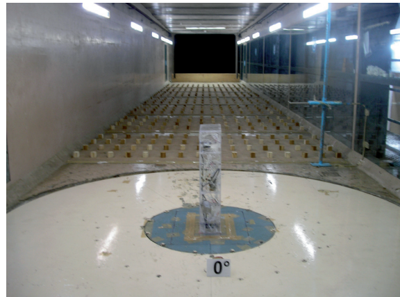
Rectangular Building Model (1:2:5) inside Wind Tunnel
