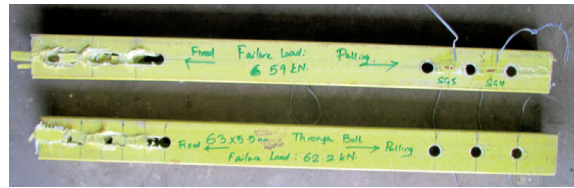
Fig. 1. Tested specimen (63 x 5.5mm) square hollow section
