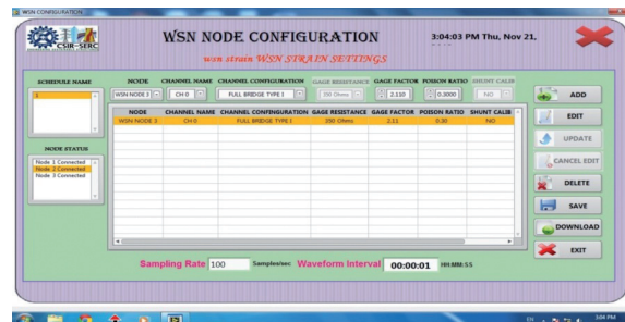
Fig. 4 Screenshot of the developed software for wireless sensor network
