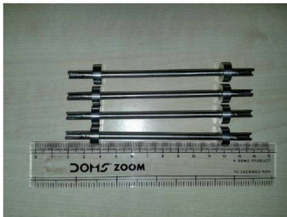
Fig. 11 Sensor housing for embeddable strain sensor array
