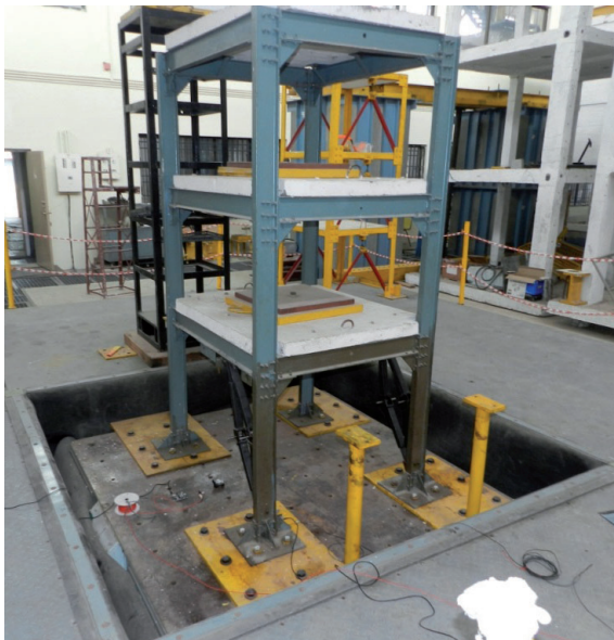
Fig. 20 Test setup on shake table for evaluation of wireless sensors
