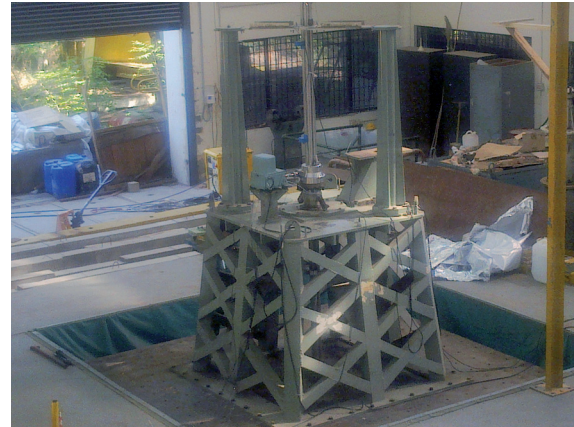
Vibration studies on CRDMs (EPS 1) using 4mx4m Tri-axial Shake-Table Facility at ASTaR Laboratory
