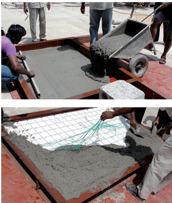
Fig.1 Casting sequence of EPS test specimens
