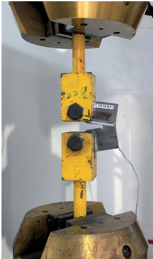
Fig. 8 Close-up view of C(T) specimen after failure
