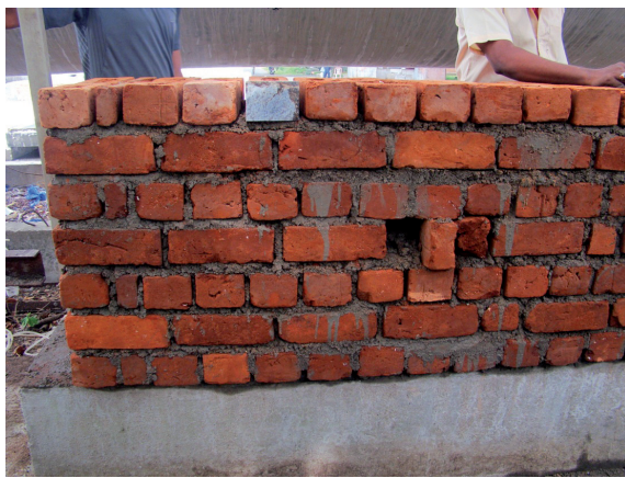
Fig. 22 Typical brick wall specimen with different variables such as materials, voids, etc.
