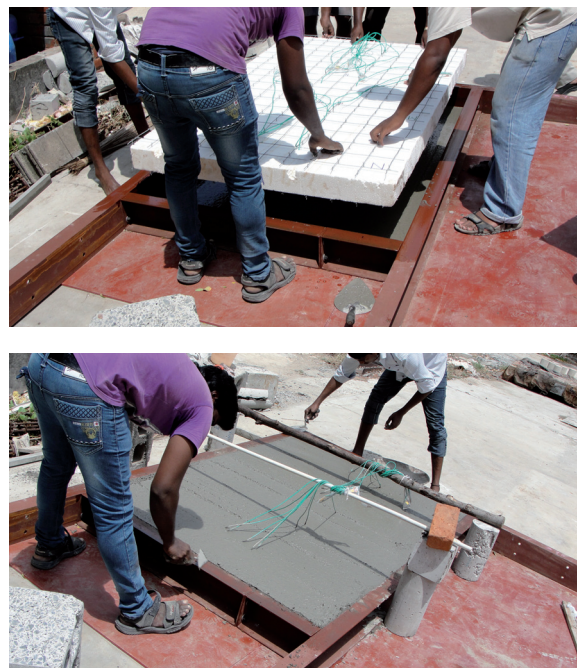
Fig.1 Casting sequence of EPS test specimens
