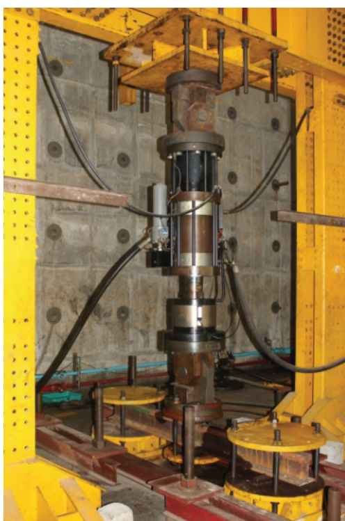
Fatigue test on a typical welded rail joint
