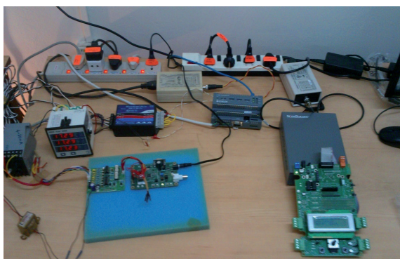
Fig. 17 Power line working setup with energy nodes, physical node and internet server module
