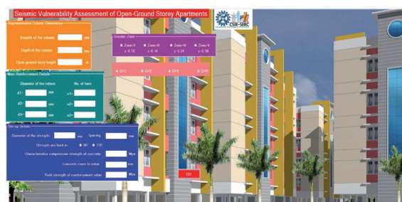
Fig. 2 Graphical user interface of the developed software to assess vulnerability of Open Ground Storey (OGS) buildings
