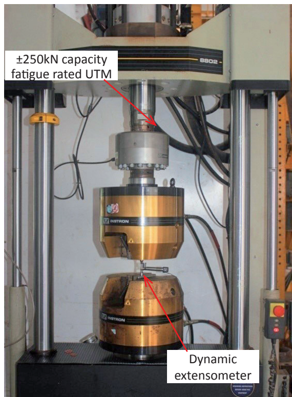
Fig. 1 Set-up for strain-controlled fatigue test on M50 alloy steel
