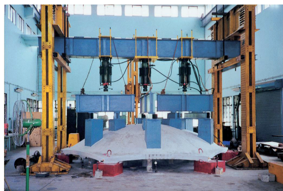
Prototype bubble-type Dome unit undergoing strength evaluation test
