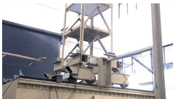
Fig. 3 Half-scale model of a reinforced concrete open ground storey building for performing shake table experimental investigations to establish soft storey effect including torsional effect
