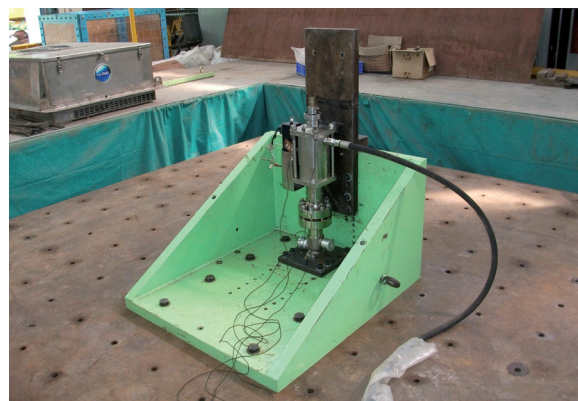
Seismic qualification studies on control valve (S14) using 2mx2m Tri-axial shake-table facility
