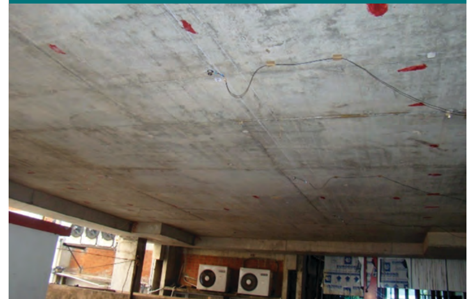
Accelerometer instrumentation of ELB of CSIR-SERC during construction stage for vibration measurement
