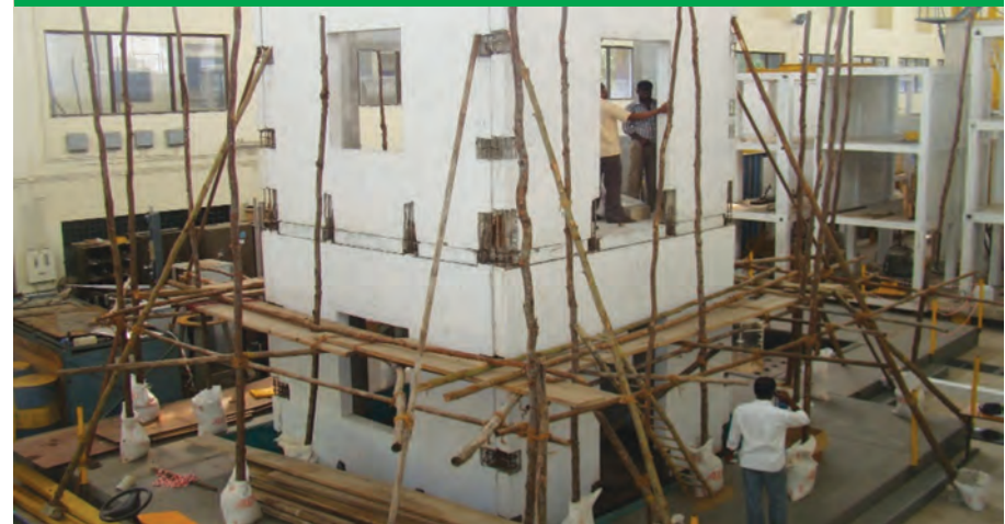
View of precast wall and floor panels assemble for (G+1) building on shake table for seismic test
