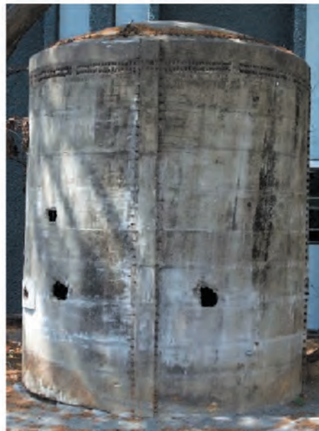
The world's first scaled micro-concrete containment vessel model
