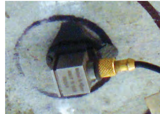
Accelerometer instrumentation of ELB of CSIR-SERC during construction stage for vibration measurement
