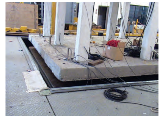
Model building on base isolator
