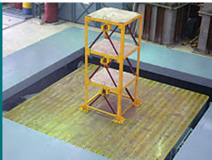
4m x 4m and 2m x 2m tri-axial shake table facilities
