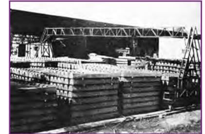
Pre-stressed concrete mono block railway sleepers made at Kosikalan, U.P, with the know-how developed by CSIR-SERC
