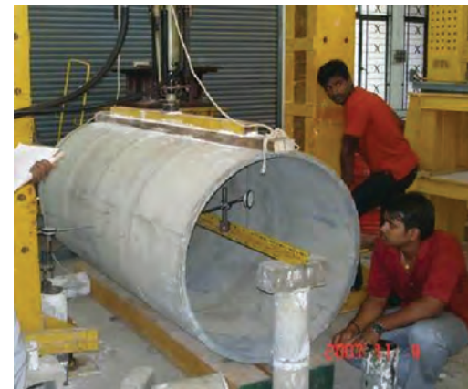
Circular Specimen under 3-edge load
