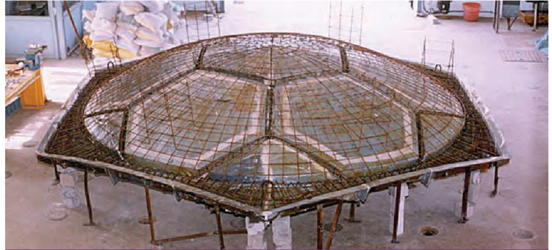
Prototype Bubble-type Dome Unit undergoing Strength Evaluation Test
