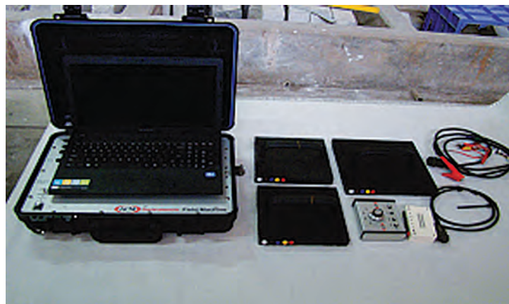
AC impedance based corrosion measurement system
