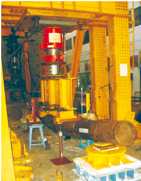
A close-up of the instrumentation during ratcheting test
