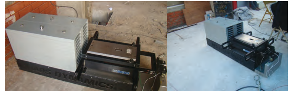
APS Dynamics Model 400 ELECTRO-SEIS shaker with additional reaction masses for testing in horizontal excitation
