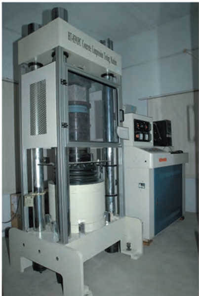
3000 kN capacity servo control Compression Testing Machine
