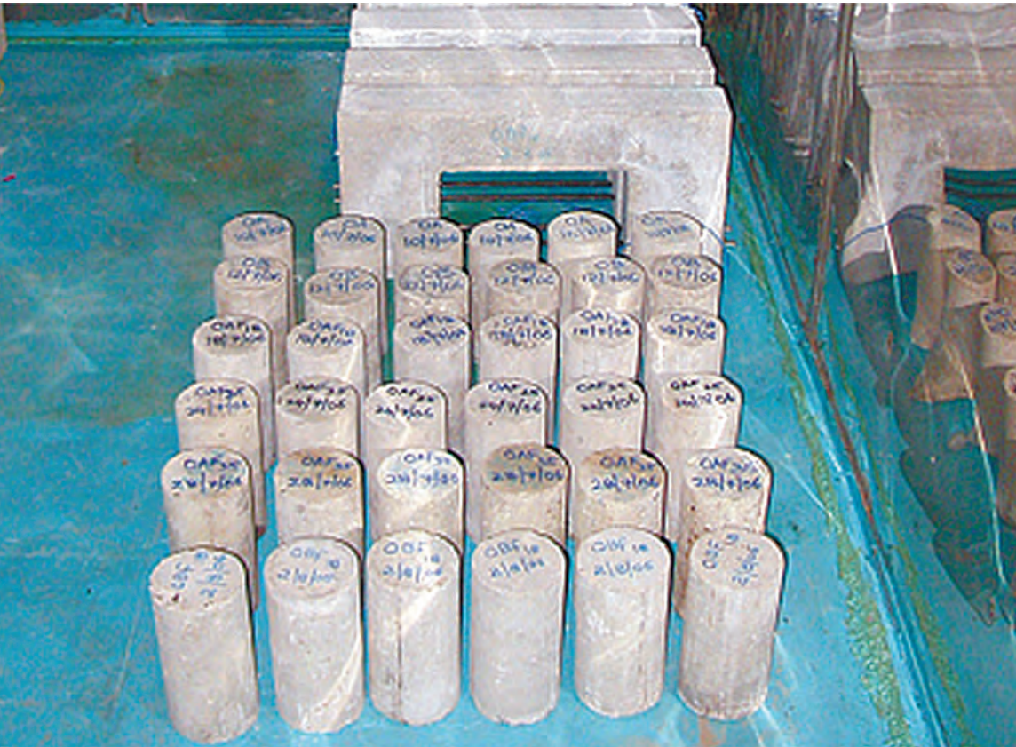
A view of test specimens exposed to accelerated carbonation in walk-in type carbonation chamber
