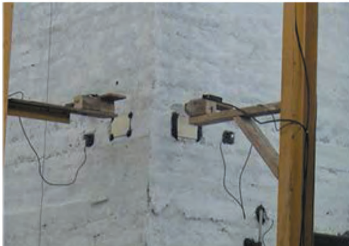
Acceleration pickups and non-contact laser-based displacement sensors
