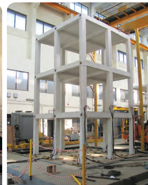
Shake table test on base isolated building
