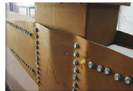
Experiments on Self-drilling screw lap joint
