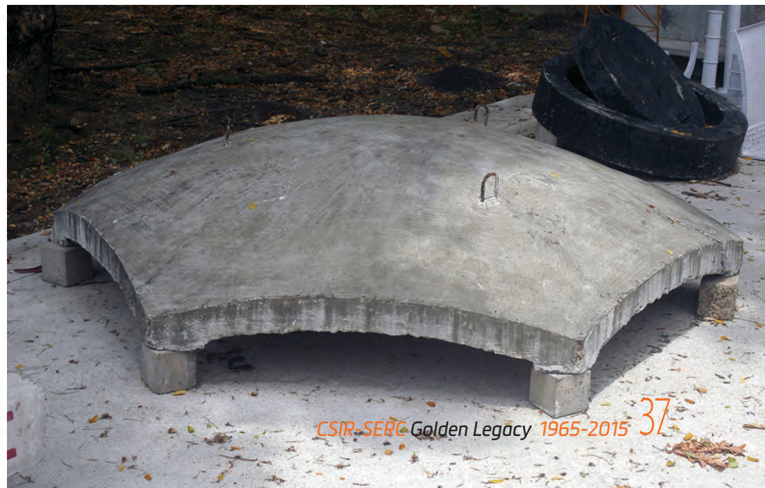
The world's first scaled micro-concrete containment vessel model
