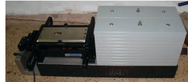
Shaker model 400 with 4001 0.5Hz Horizontal Operation reaction mass system
