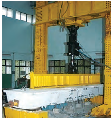
Static test up for epoxy jointed segmental box girder
