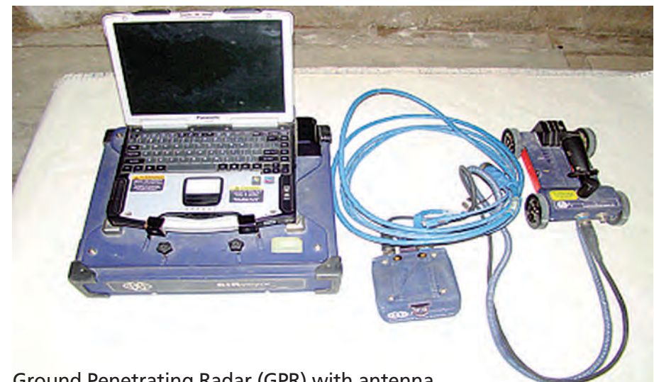
Ground Penetrating Radar (GPR) with antenna
