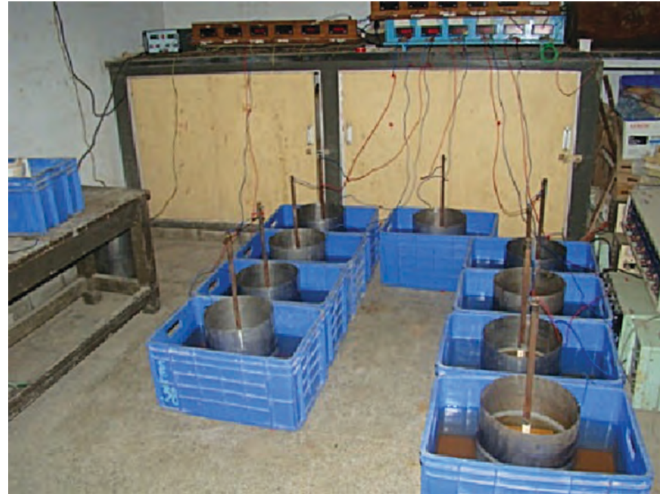
Pull-out specimens under accelerated corrosive conditions
