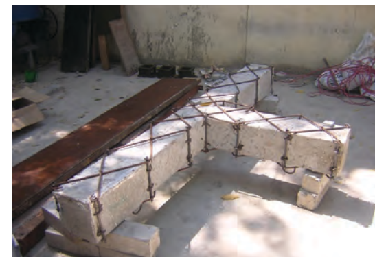
Reinforcement Details for Concrete Jacketing
