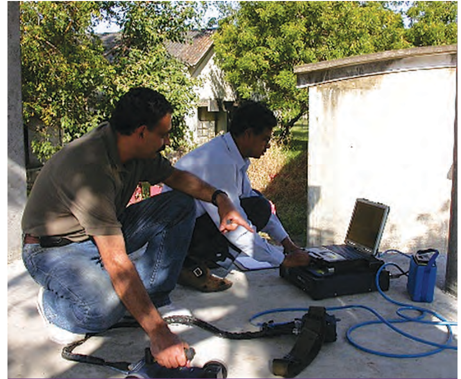
Measurement with 1.6GHz antenna
