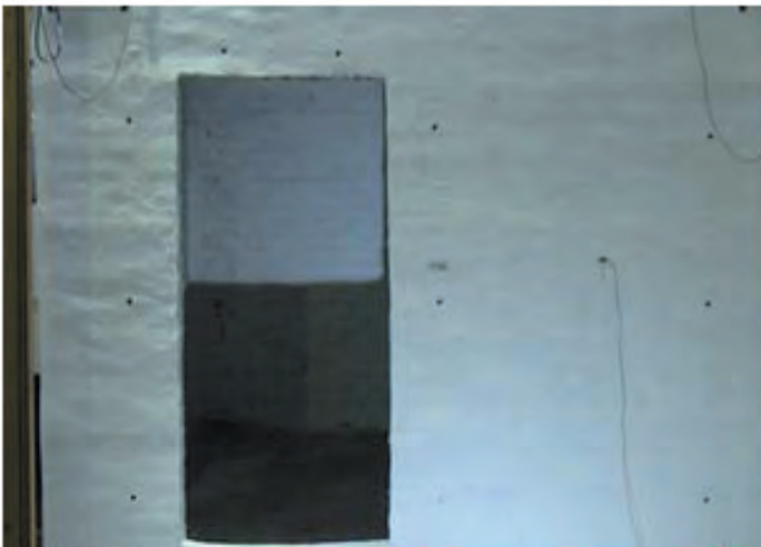
Markers on the test structure, for displacement measurement from image processing
