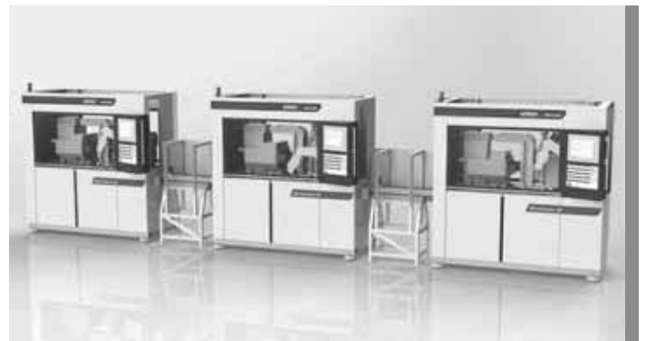
Example of special process: Three-component micro injection moulding machinery (courtesy of FOTEC Forschungs- und Technologietransfer GmbH and Wittmann Battenfeld GmbH).
