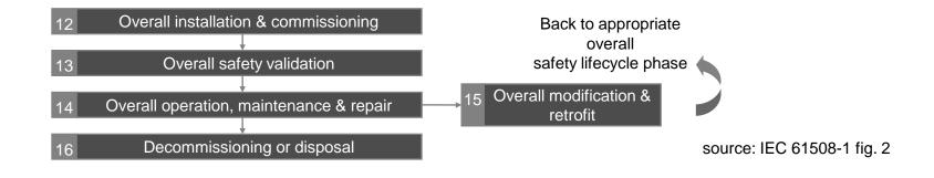
Prior to modifying the SIS functions on a running installation, a hazard and risk analysis needs to be carried out >> Management of Change procedure
